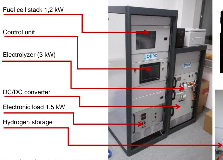
Electrolyzer single cell test station
